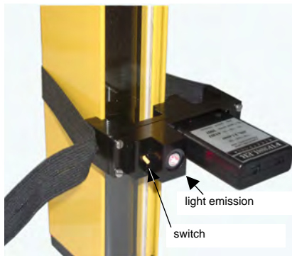
Fixation on XLVT housing
