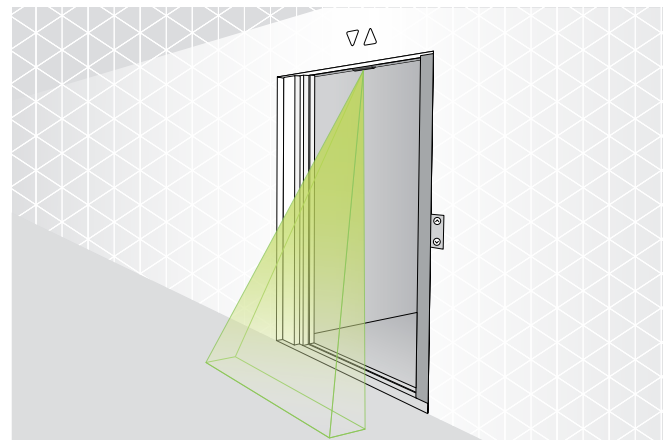
IMS 100 NT - center-mounted for center-opening doors
